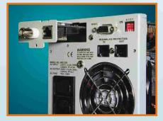
A true RS232 communication port is supplied as standard with each UPS. This can be used with the software provided or an external SNMP adapter. The Options slot allows further flexibility in network configuration. Three cards are available: an internal SNMP card, AS400 card or a true relay card to provide isolated contacts for industrial and remote alarm panel applications.
